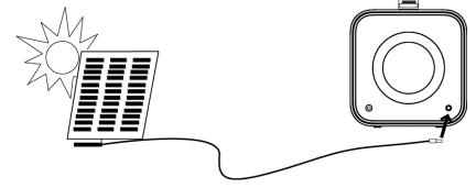
**Note**: When the sunlight is not strong enough to support continuous input charging, please press the USB power switch to trigger the system.
