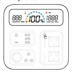
5 .UA1100 supports input and output charging simultaneously(UPS), the screen will show both charging status as well as various function modes. When charging and discharging at the same time, overheat temperature protection is based on the charging temperature.
