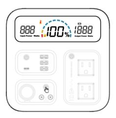
3 . Long press LED switch button for 1.5 seconds to light on the LED, letters LED will show up on the screen; long press it for 1.5S again to switch off the LED light.
