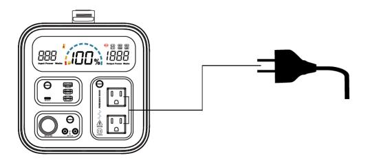
**Note:** When the AC port is not in use, turn off the AC power button to conserve power.
