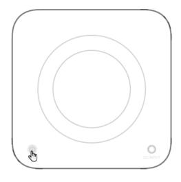
4 . Long press AC switch button for 1.5 seconds to start AC function, AC mode will show up on the screen; long press it for 1.5S again to shut the function. Long press it for over 3S to shut the whole generator.
