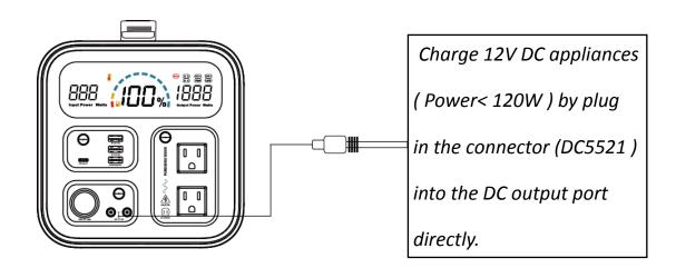
**Note**: The DC output of this power station is approx constant 12.8V. The max output current is 10A. Please make sure your appliance can match this voltage.
