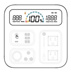
2 . Long press DC switch button for 1.5 seconds to start DC function, DC mode will show up on the screen; long press it for 1.5S again to shut the function. Long press it for over 3S to shut the whole generator.
